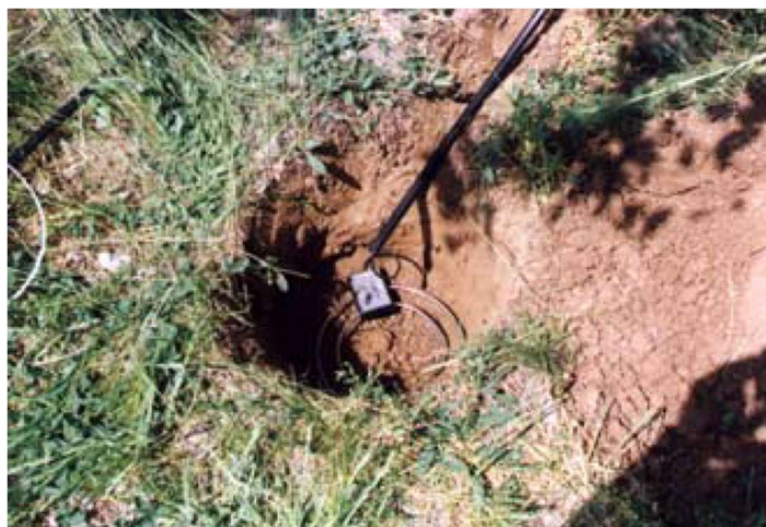
Image 6: Example of a hole for sensor placement
